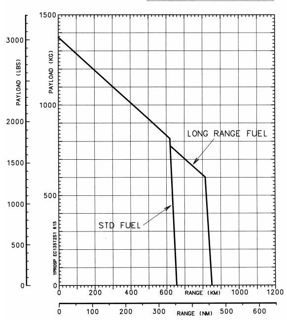
PAYLOAD RANGE DIAGRAM (STD FUEL 560KG)
